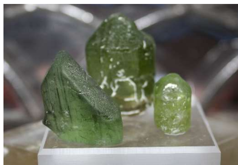
Figure 6. Variants of peridot crystals. Although the top peaked terminations are obvious, most peridot crystals show a rounding or softness of the edges and terminations
