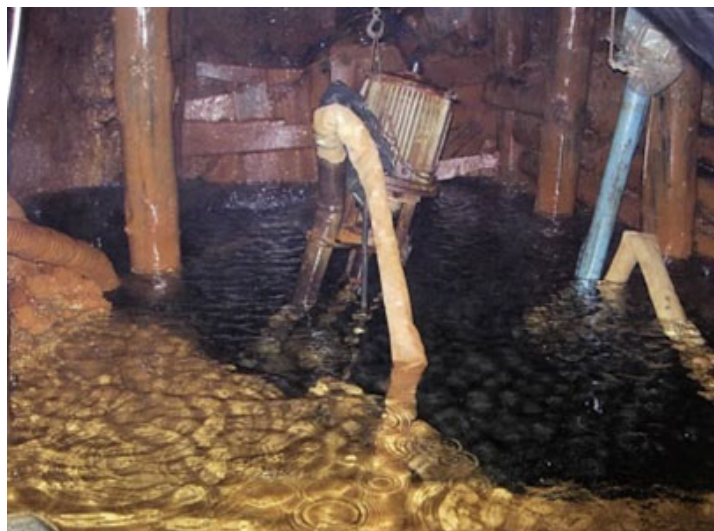
Figure 22 Constant pumping of water was needed in pegmatite 364 to avoid pocket flooding and risk to miners
