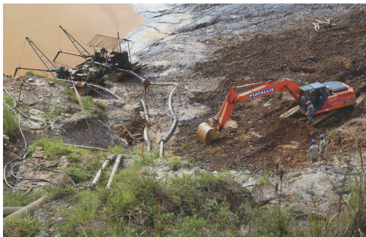
Figure 17. Lavra do Capao. A backhoe works the country rock. The water pumps and hoses can be seen on the left of the photo
