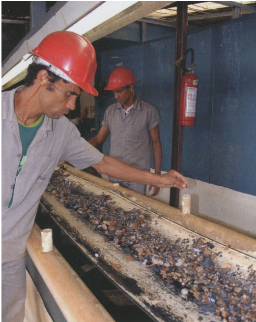
Figure 19. Lavro do Capao. A worker at the conveyor belt places a topaz into the capture system tubing on the sides of the conveyor. The topazes are then carried off to the owner or overseer for examination
